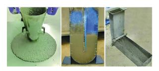
A concrete mix can only be classified as Self Compacting Concrete (SCC) if the same is able to flow under its own weight and completely fill the formwork, even in the presence of dense reinforcement, without the need of any vibration, whilst maintaining homogeneity. More technically, SCC should meet the requirements for filling ability, passing ability and segregation resistance, as mentioned in below table:
